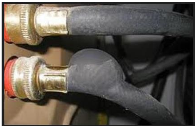
Unbraided rubber hoses under pressure.
